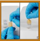
seal from the reagent cap and push the cap onto the sample tube until the cap is flush with the tube top.
