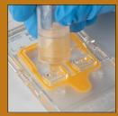
e. Twist off the cap tab and dispense the entire tube of solution into the applicable cartridge port (left or right). Then, repeat ear swab steps 2a-2e for the right ear swab, using the other sample tube, reagent cap, and cartridge port.
