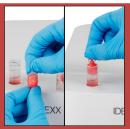
c. Pull to remove the foil seal from the reagent cap and push the cap onto the sample tube until the cap is flush with the tube top.
