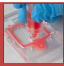
e. Twist off the cap tab and dispense 6 drops of the solution into the cartridge
