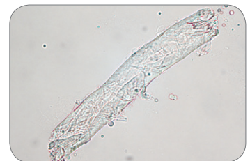
Figure 24 Contaminant fragmented fiber
